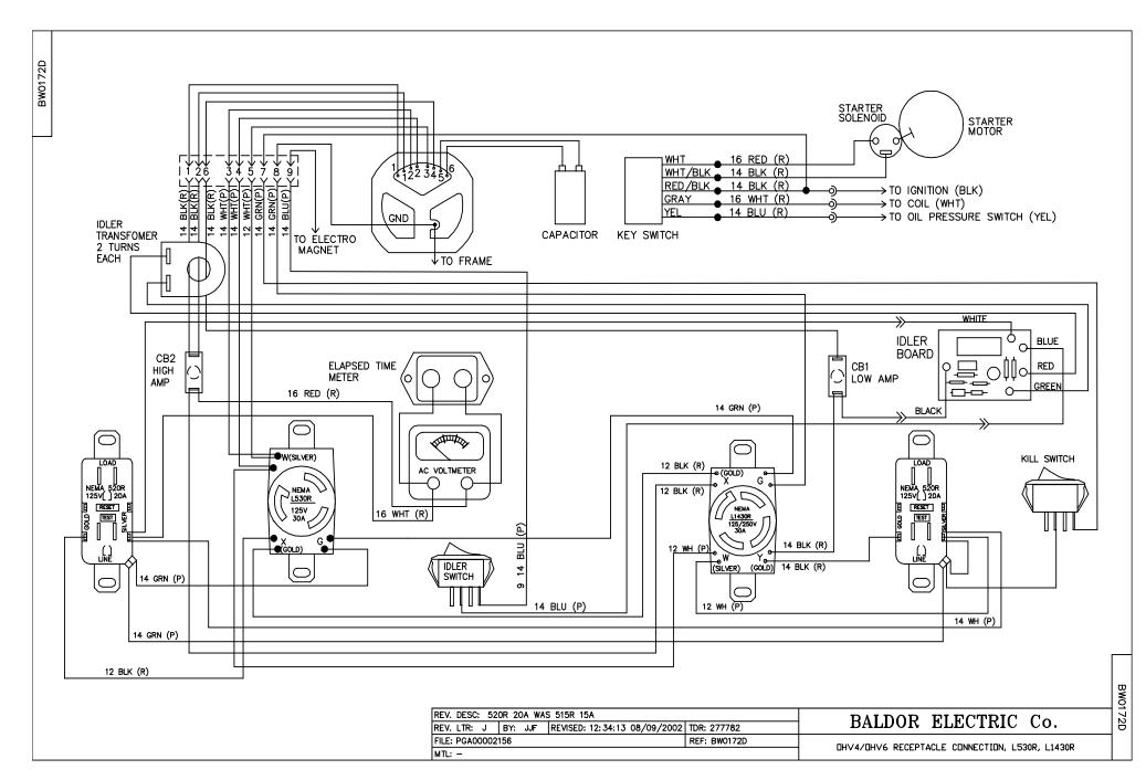
Wiring Diagram OHV40, OHV50, OHV60
